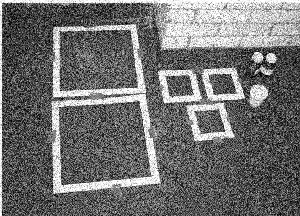
Photo 6: Common Space Floor Wipe Template Set up
